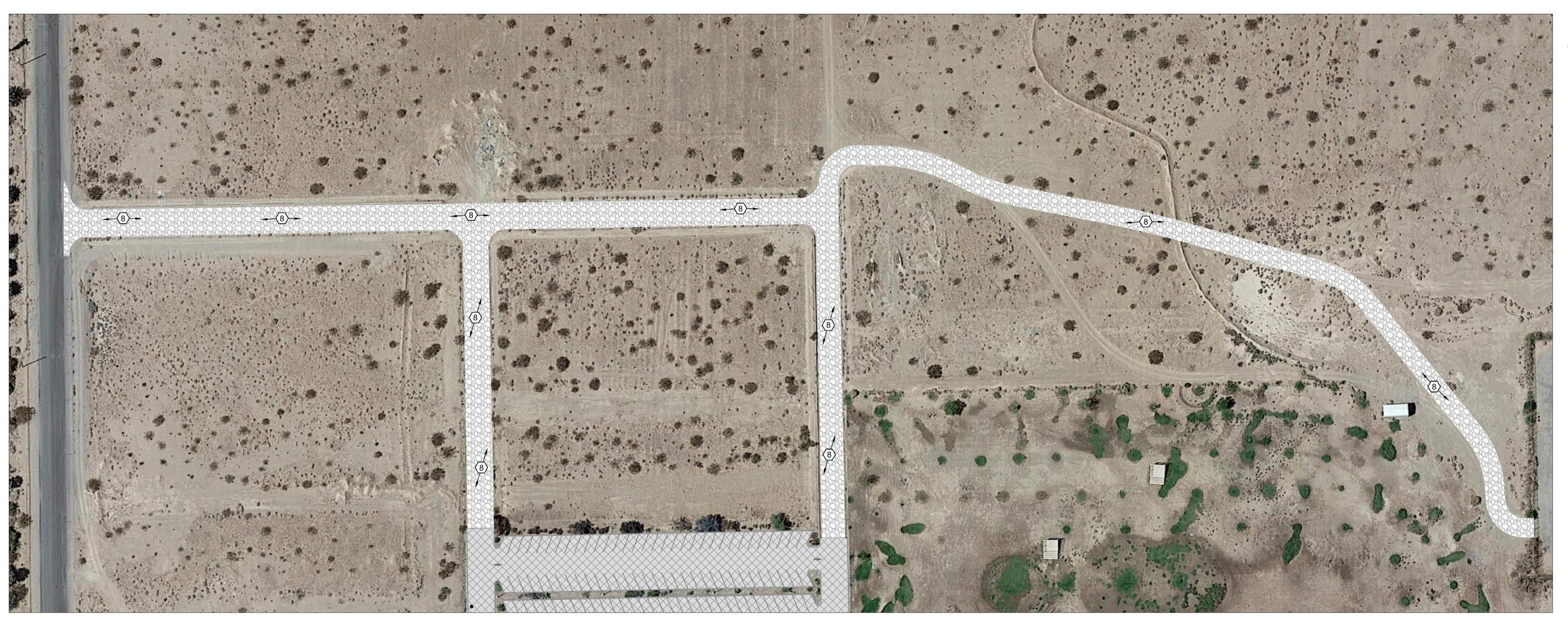
(8) INSTALL 3-INCHES OF THE PARKING LOT A.C. GRINDINGS AS ILLUSTRATED ON SHEET 12 OF THE IMPROVEMENTS PLANS. COMPACT A.C. GRINDINGS MATERIAL TO 90 PERCENT MAXIMUM DENSITY PER ASTM D-1557.
